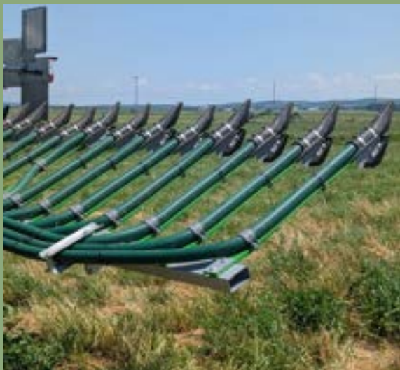
A "trailing shoe" liquid manure spreader attachment, to spread manure close to plant roots instead of on foliage
