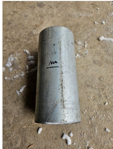
Figure 3. The single ring infiltrometer, with 8.5 cm diameter and 20 cm long, used for the experiment.
