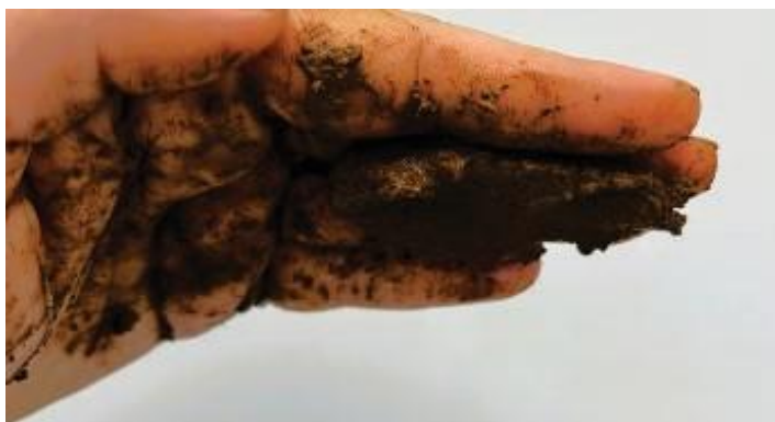
Figure 4. Soil wetness for determining texture. The soil should stick to your fingers when inverted but not drip with water.
