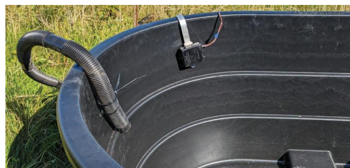
A marine switch powers a bilge pump which will draw water into the tub.
