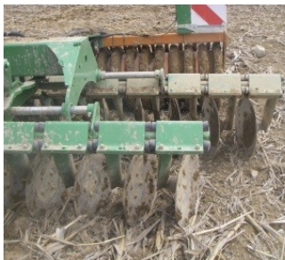
Riordon: showing Catros disc angle set.
